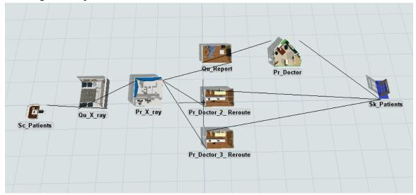
Figure 1. Model view in FlexSim interface
