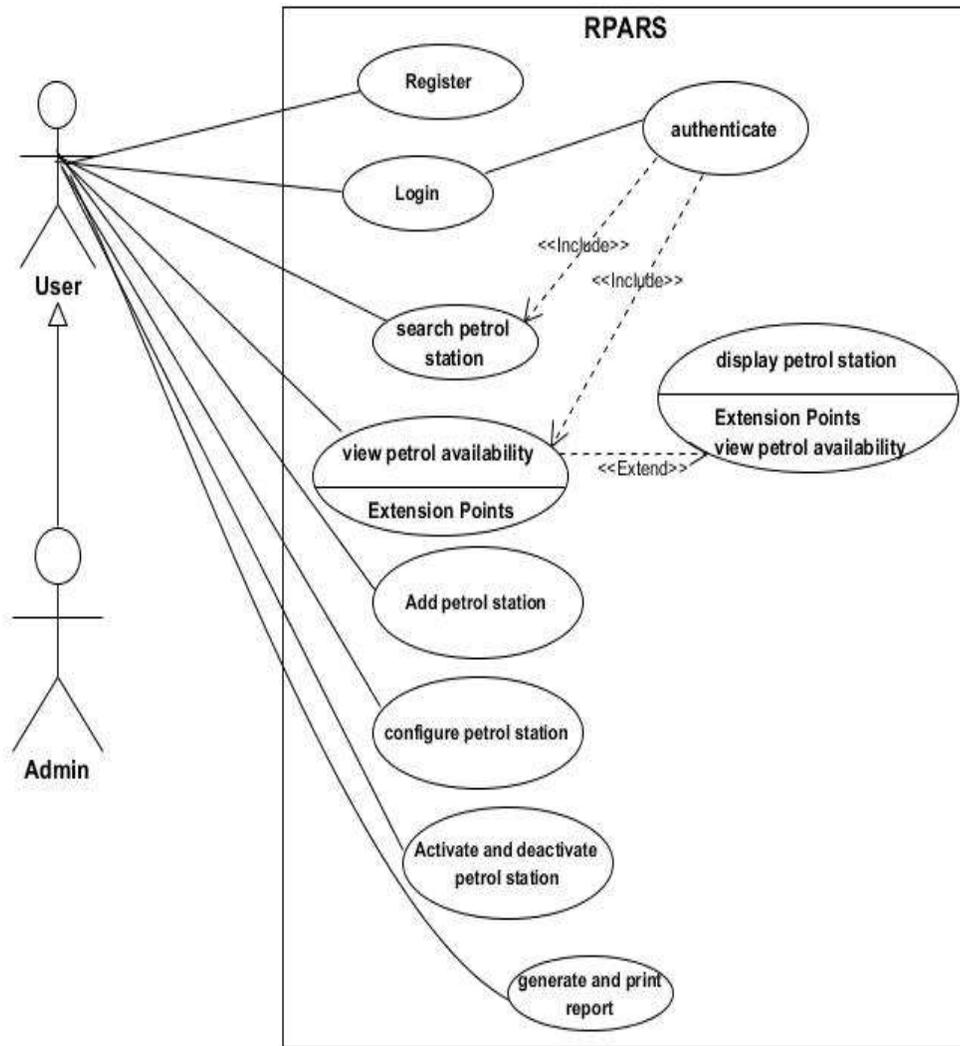
Figure 2: Use Case diagram of the RPARS
